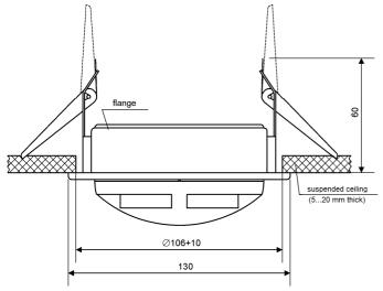
• Select the place on the ceiling to secure the detector.
