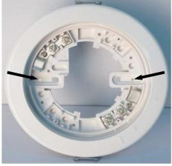
• Align the slotted holes of the base with holes on the flange, insert screws provided into holes, and fix the base into the flange.
