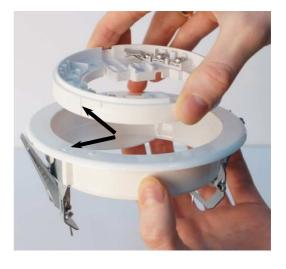
② Pass the wiring through the mounting hole. Insert the detector mounting base into the flange aligning the longer match mark on the base with the longer match mark on the flange.
