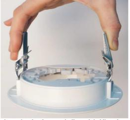
• Lift the spring brackets vertically and holding them in this position insert the flange into the mounting hole; then release the brackets. Connect wiring to the terminals as per the project design and as described in the detector instruction manual.
