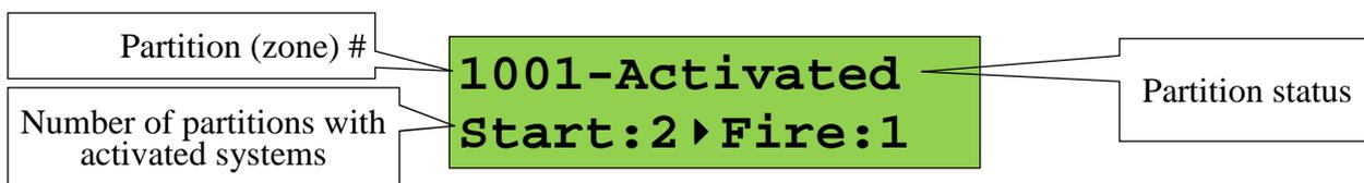
In case of pre-activation, the display shows the Start countdown for the zone where the activation will happen first.
