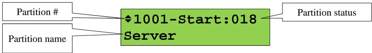
To navigate between zones where release/start signal is activated, please use  $\blacktriangleright$   $\blacktriangleleft$ . The  $\blacktriangleright$  key pages partitions in the order they were activated, the  $\blacktriangleleft$  button does it in the reverse order.
