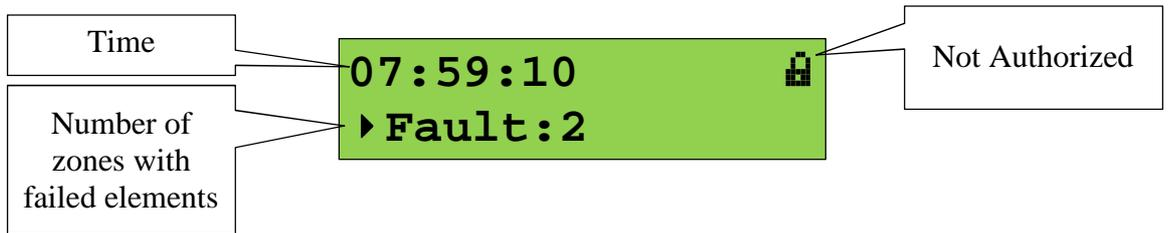
To view faulty elements, please press the **▶** button (**◀ ▶** are used to select to view Starts, Faults, Alarms, Stops, Faults, and Disablements). It will show info on the partition first gone to the fault status:
