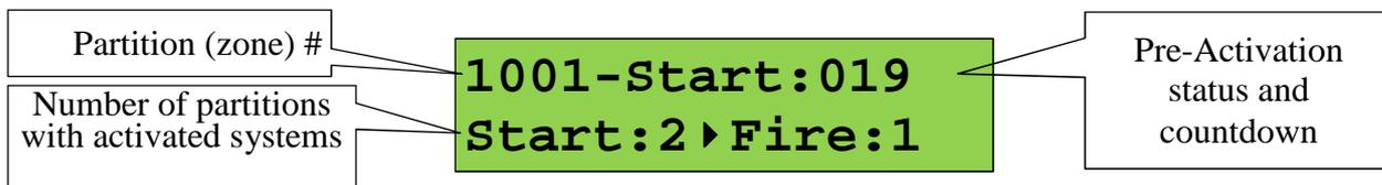
An activation signal in the zone (e.g VA immediate manual activation) can be initiated manually by pressing the **START** button, the abortion of the activated system can be done by pressing the **STOP** button. These operations as well as other available commands can be committed through the contextual menu. To open this menu, please press **≡◊**.
